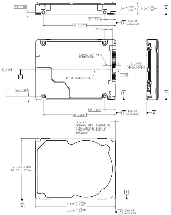
Figure 9. Mounting configuration dimensions
